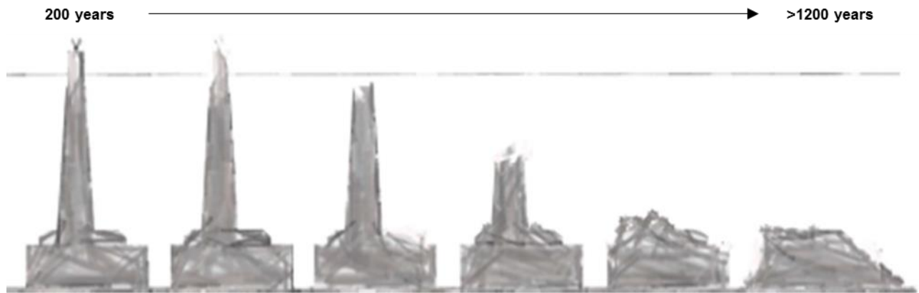
Figure 2.20 Long term degradation of the Dunlin Alpha substructure over time.
