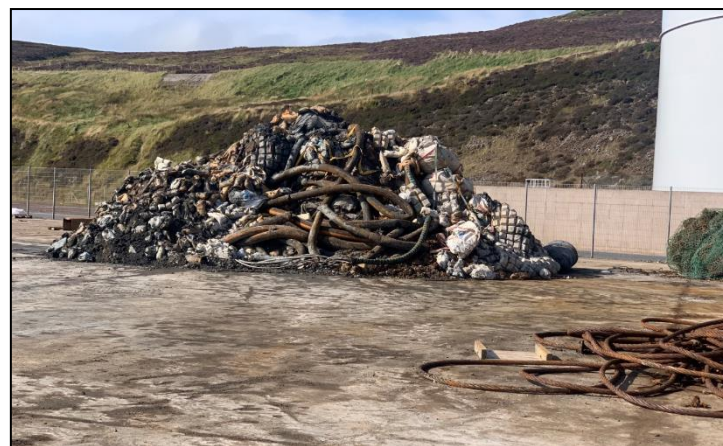
Mixed Sand / Grout / Mattress Deposits Recovered for Landfill (Note flexible hose and umbilical were not recovered by Fairfield)
