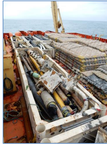
Infield Jumpers and Flowlines Recovered
