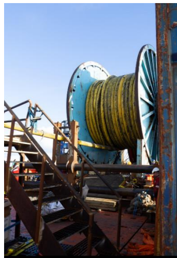
Normand Clipper Reverse Reeling 8" Water Injection Line, PL735A
