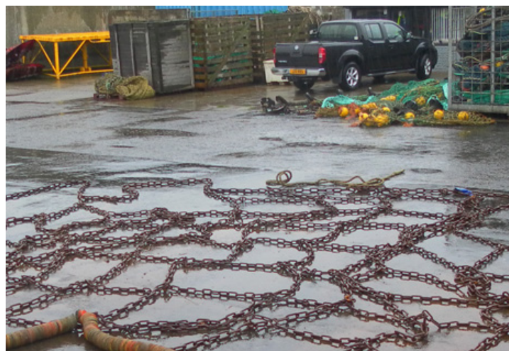
Figure 2.11 Chain mat shown on the quayside (system shown from SFF, 2016)
