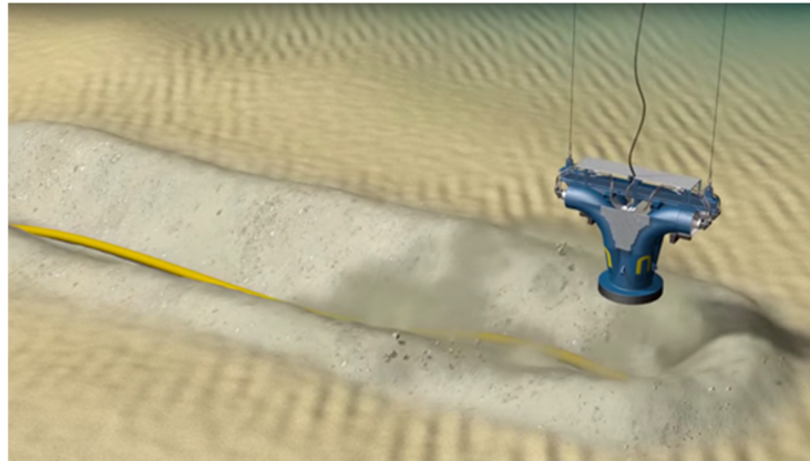
Figure 2.8 Illustration of a pipeline being exposed by a jet of water from a mass flow excavator (system shown from N Sea, 2017)
