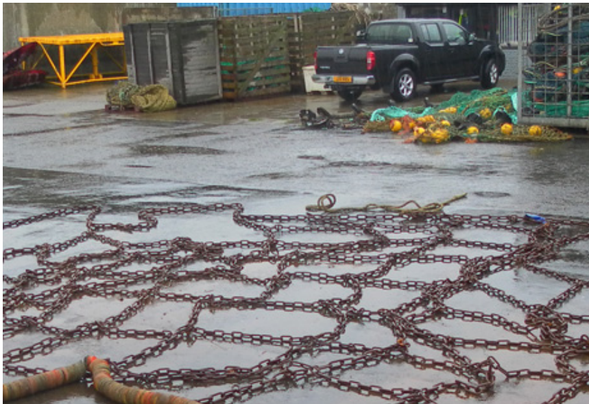
Figure 2.12 Chain mat shown on the quayside (system shown from SFF, 2016)
