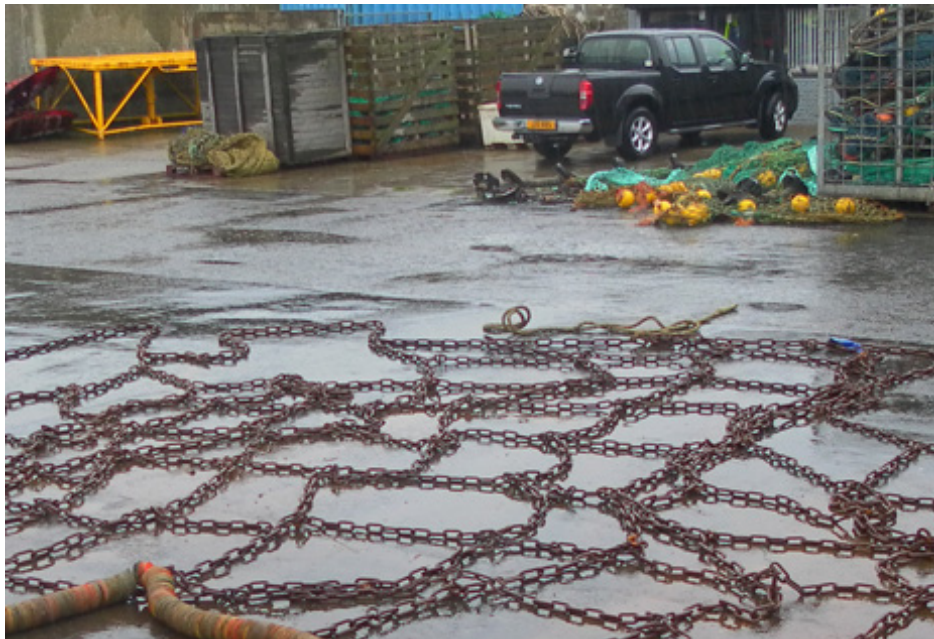
Figure 2.10 Chain mat shown on the quayside (system shown from SFF, 2016)
